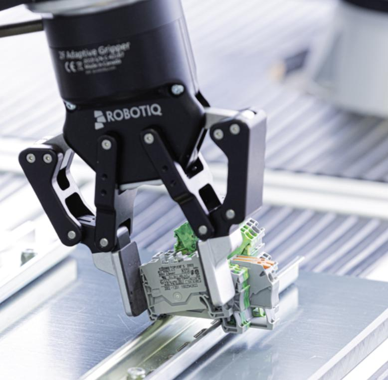
*Parts can be gently inserted or snapped into place with great efficiency, e.g. such as when mounting components on top hat rails for a control cabinet.*
